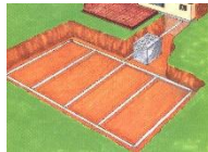
Septic tank with a drain field
